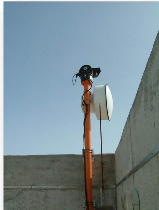
Figure 9: Close-up of system (IR payload only) with optional integrated RF system.
