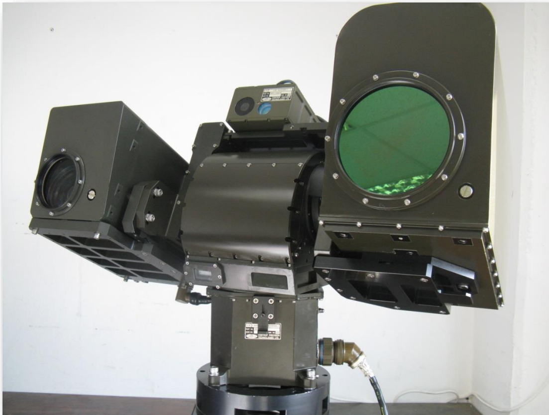
Figure 1: INTERCEPTOR System Payload. IR camera is located on the right-hand side of the system. CCD camera on the left-hand side. Long-range laser range finder is located on the top portion of the unit. All components are separately removable and customizable.
